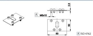
ISO 2 - Closing plate for sub-base 2 material: steel weight: 0,050 Kg (for all sub-base versions)
