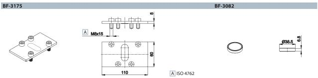
ISO 3 - Closing plate for sub-base 3 material: steel weight: 0,080 Kg (for all sub-base versions)
